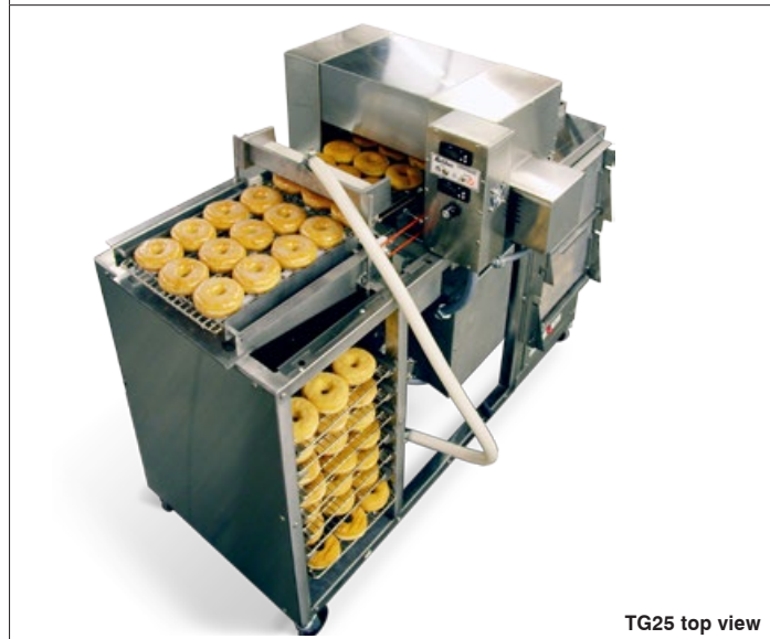
Thermoglaze TG25. 8-shelf Thermolizer is shown at right (with door open). Storage shelves are shown at left.
