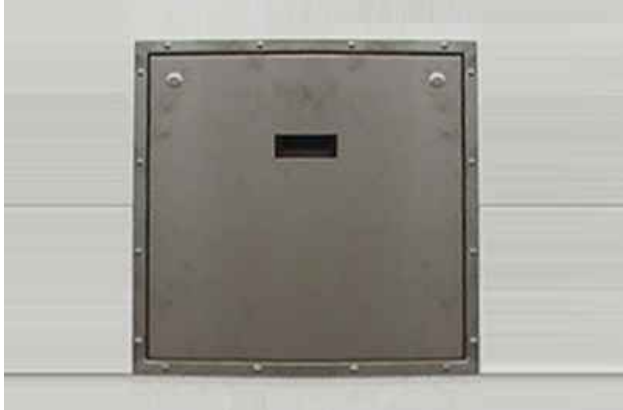
Along the oven at the opposite of control side, for cleaning and maintenance purposes.
