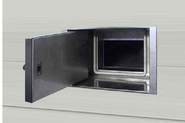
Along the oven at the control side, for checking the baking progress. Provided with mobile lamp for inspection.
