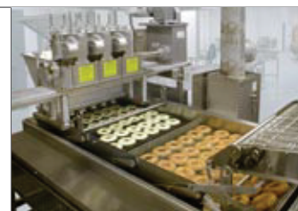
Century C6-16 — 6 ft. long fryer, 4 standard donuts per pocket, frying raised donuts (right). Gas and electric models available.
