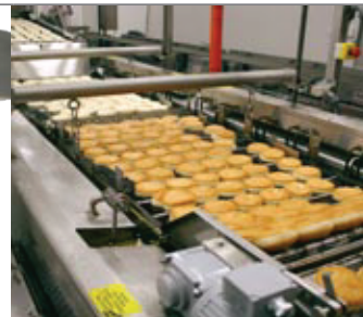
Century C10-24 — 10 ft. fryer, 6 standard donuts per pocket, shown frying raised donuts. Gas and electric models available. Conveyor hoist is standard. (Hood optional)
