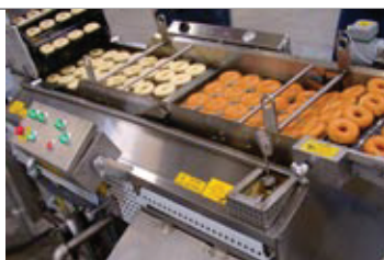
Century C6-16 — 6 ft. long fryer, 4 standard donuts per pocket, frying raised donuts (right). Gas and electric models available.
