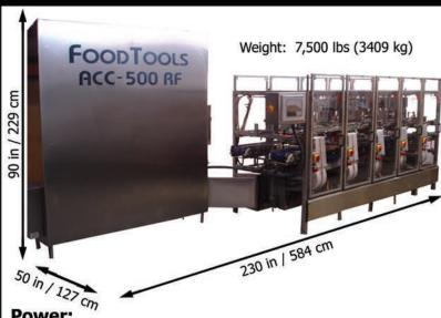
Power: Compressed Air 40 CFM @ 90 PSI Electric 480V/60/3 Phase, 60A
