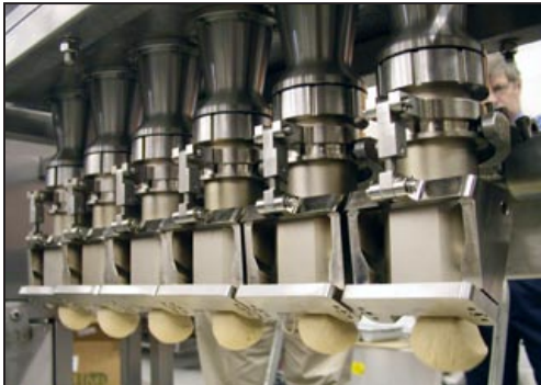
◀ Belshaw Pressure Cutter producing shells (Bismarcks)
