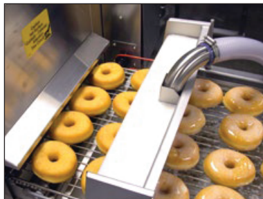
TG50 glazer in operation
