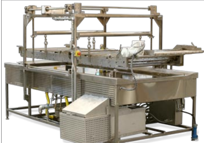
Century C10-36 — 10 ft. fryer, with 36" width for 8 donuts per pocket. Gas only with conveyor hoist standard. All models C10-24 and higher (gas and electric) incorporate this same overall design.
