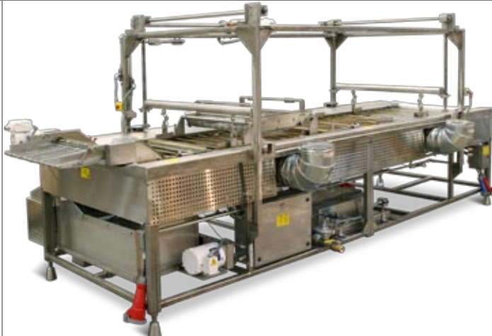
Century C14-24 14 ft. fryer, holds 6 donuts per pocket, with conveyor hoist standard. Century C14-36G 14 ft. gas only fryer, holding 8 donuts per pocket, with conveyor hoist
