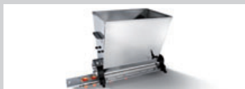
Roller head for hard dough
